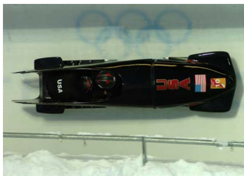
Figure 5.8 From racing cars to bobsled racers, aerodynamic shaping is crucial to achieving top speeds. Bobsleds are designed for speed. They are shaped like a bullet with tapered fins. (credit: U.S. Army, via Wikimedia Commons)
