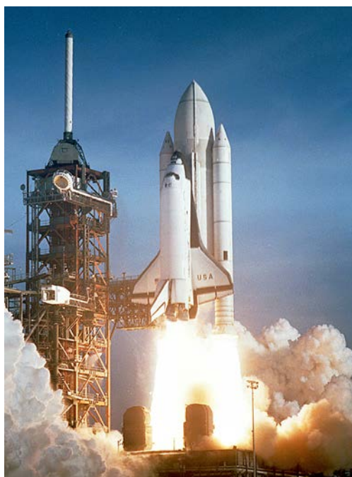
Figure 8.17 The space shuttle had a number of reusable parts. Solid fuel boosters on either side were recovered and refueled after each flight, and the entire orbiter returned to Earth for use in subsequent flights. The large liquid fuel tank was expended. The space shuttle was a complex assemblage of technologies, employing both solid and liquid fuel and pioneering ceramic tiles as reentry heat shields. As a result, it permitted multiple launches as opposed to single-use rockets. (credit: NASA)
