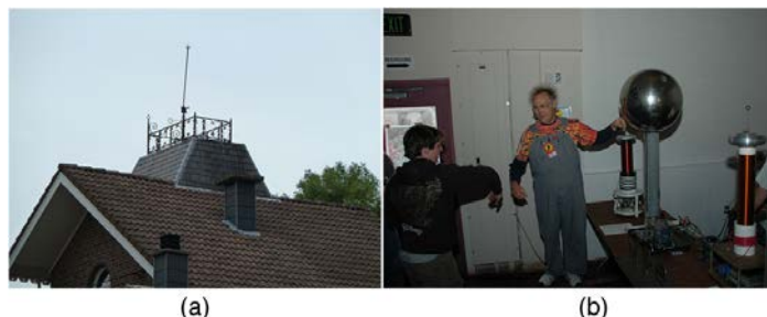
Figure 18.25 (a) A lightning rod is pointed to facilitate the transfer of charge. (credit: Romaine, Wikimedia Commons) (b) This Van de Graaff generator has a smooth surface with a large radius of curvature to prevent the transfer of charge and allow a large voltage to be generated. The mutual repulsion of like charges is evident in the person's hair while touching the metal sphere. (credit: Jon 'ShakataGaNai' Davis/Wikimedia Commons).
