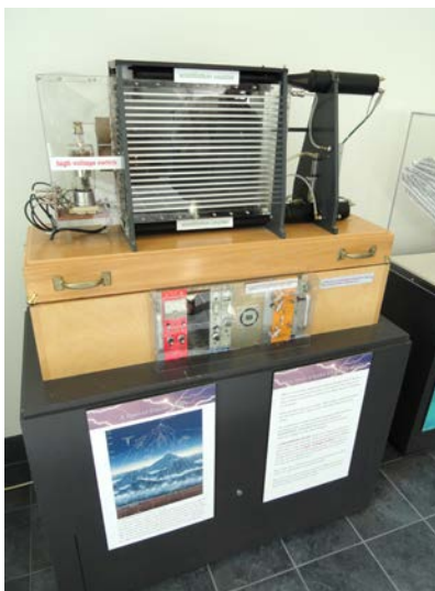
Figure 19.8 A spark chamber is used to trace the paths of high-energy particles. Ionization created by the particles as they pass through the gas between the plates allows a spark to jump. The sparks are perpendicular to the plates, following electric field lines between them. The potential difference between adjacent plates is not high enough to cause sparks without the ionization produced by particles from accelerator experiments (or cosmic rays). (credit: Daderot, Wikimedia Commons)
