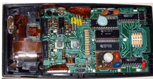
Figure 19.30 Energy stored in the large capacitor is used to preserve the memory of an electronic calculator when its batteries are charged. (credit: Kucharek, Wikimedia Commons)
