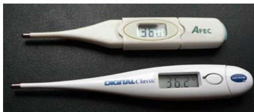
Figure 20.15 These familiar thermometers are based on the automated measurement of a thermistor's temperature-dependent resistance. (credit: Biol, Wikimedia Commons)
