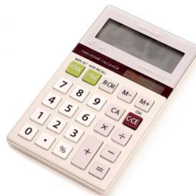
Figure 20.43 The strip of solar cells just above the keys of this calculator convert light to electricity to supply its energy needs. (credit: Evan-Amos, Wikimedia Commons)
