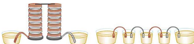
Figure 21.18 Batteries are multiple connections of individual cells, as shown in this modern rendition of an old print. Single cells, such as AA or C cells, are commonly called batteries, although this is technically incorrect.
