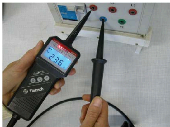
Figure 21.30 (a) To measure potential differences in this series circuit, the voltmeter (V) is placed in parallel with the voltage source or either of the resistors. Note that terminal voltage is measured between points a and b. It is not possible to connect the voltmeter directly across the emf without including its internal resistance, r . (b) A digital voltmeter in use. (credit: Messtechniker, Wikimedia Commons)
