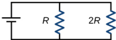
Figure 21.60 Two resistors, with resistances R and 2R are connected to a voltage source as shown in this figure. If the power dissipated in R is 10 W, what is the power dissipated in 2R ?
